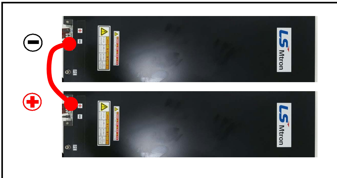
<Fig. 2> Series Connection of Modules
