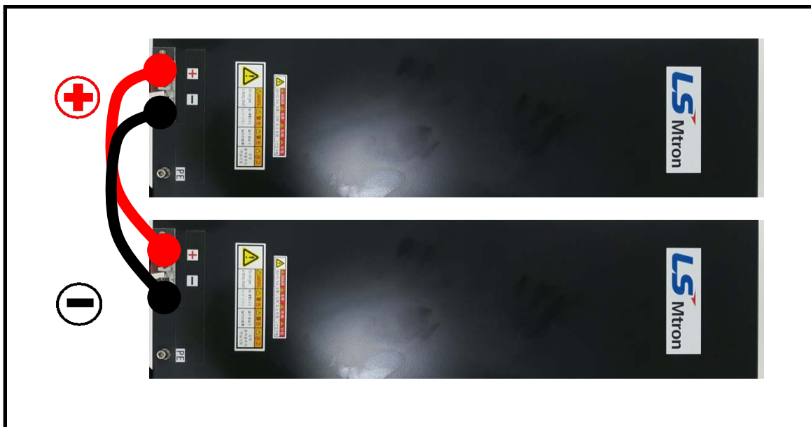
<Fig. 3> Parallel Connection of Modules.
